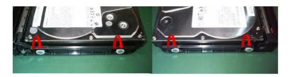
9.4 Insert HDD Carrier to case and close the cover
